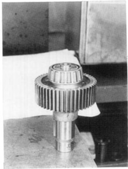
FIG. 5.1-18 Intermediate shaft removed from housing.
