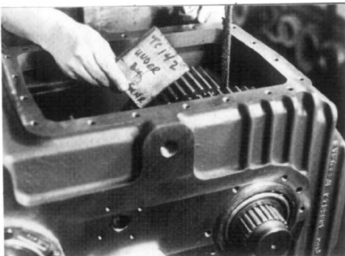
FIG. 6.4-8 Remove wooden block from under gear.
