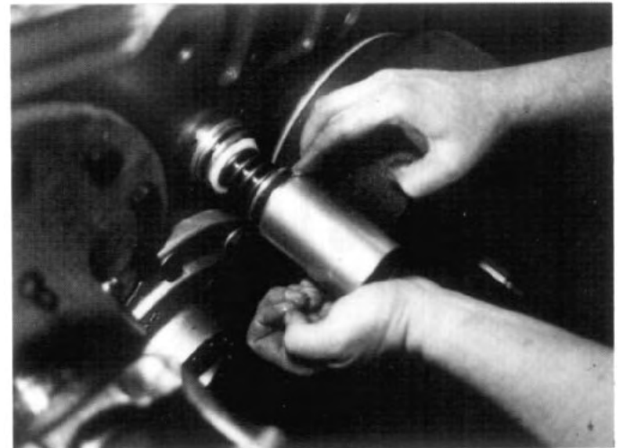
FIG. 6.6-4 Apply a liberal smear of oil and grease slurry to O-ring areas of adapter tube and piston. Presoak the piston felt seal in 30W oil overnight, and wrap into wide groove of piston. While retaining felt in groove with fingers push the cylinder tube onto the piston with the hands. Use caution not to pinch the O-ring seals.
