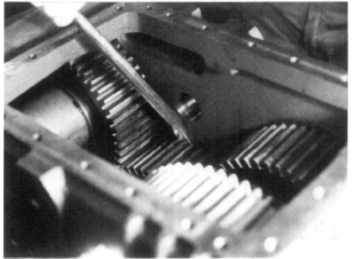
FIG. 6.5-3 With a pry bar, or other suitable tool, between the respective gear and the housing wall, use a moderate amount of hand pressure to move the shaft assembly in each direction while reading the dial indicator. Be sure the shaft is moving and not just the gear on the shaft. Vary the number of shims to provide the correct end float. All bearings on the TC-142 must have between .003 and .008 inches of end float.
