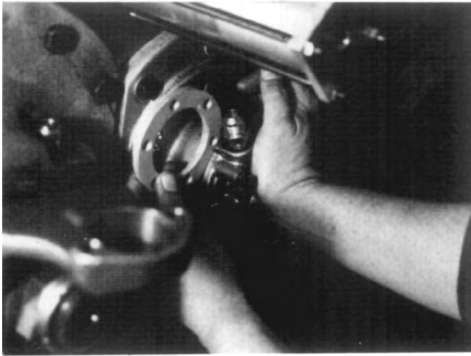
FIG. 6.8-5 Press pump end cap lightly until contact with spring, but not compression, is felt. With pack of shims measure space between cap and carrier. Remove five (5) shims from number of shims counted and assemble under cap. Once again noting that pin correctly engages shoulder slot. Leave at least 1 shim in pump assembly.
