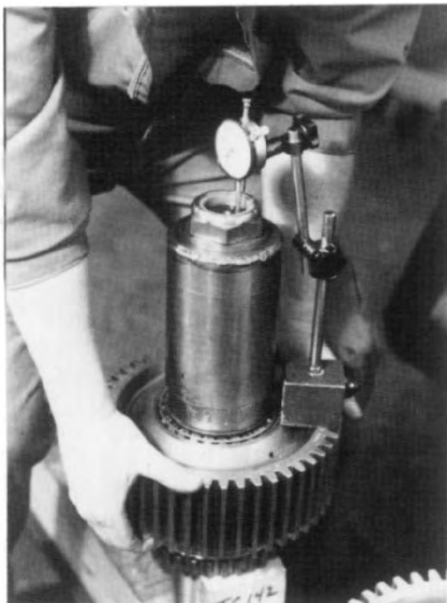
FIG. 6.3-6 Using tool number 866 649 assembled to shaft with locknut check end float with dial indicator as shown. Total end float should be .003 to .008 inches. Replace spacer between bearings with one of suitable size to provide correct end float.
