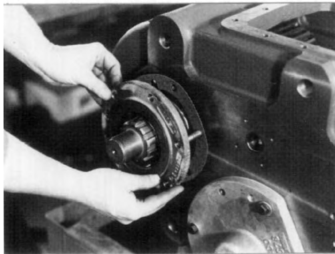
FIG. 6.2-8 Press seal into front carrier, and assemble with gasket to front of housing.
